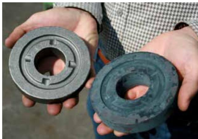
Initial state before the blast process (right) and cleaning result after the blast process (left)
