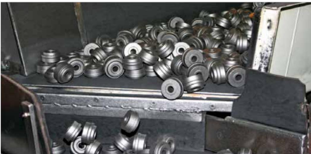
Clean parts after the blasting process. The steel abrasive specification comprises shot and grit at particular controlled hardnesses
